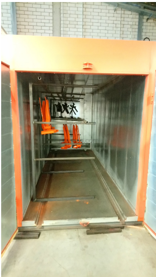
Chain conveyor / sliding doors
